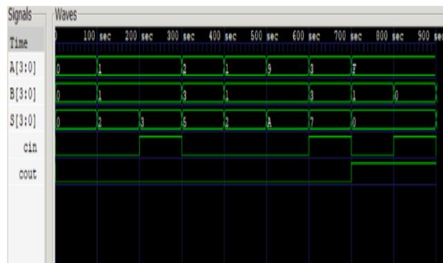
Figure 9. Waveform of Carry Save adder which shows how the addition is performed in respect to the addition
