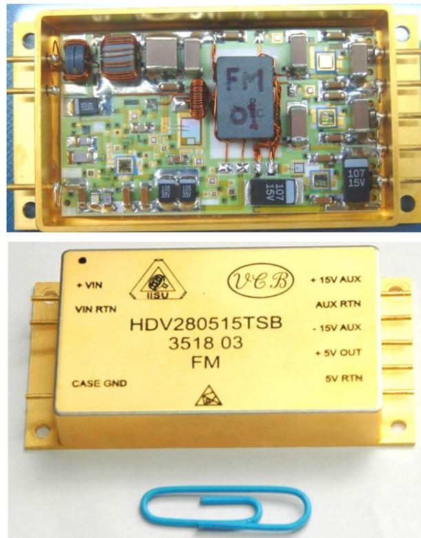
Fig. 2. Indigenous HMC DC-DC Converter with Built-in EMI filter
