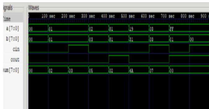
Figure 8. Waveform of Carry look ahead adder the output shows a less delay of the gates.
