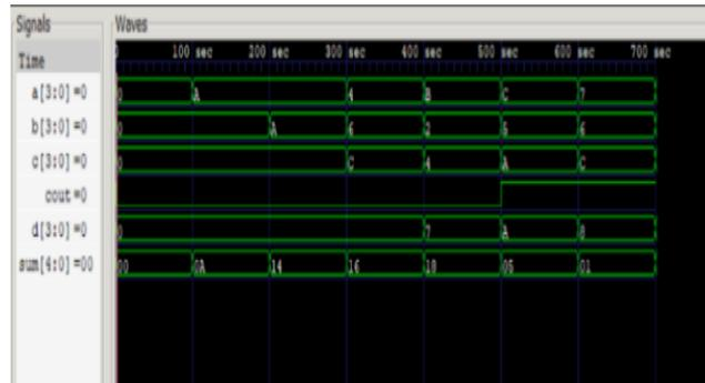
Figure 10. Waveform for Carry skip adder the output was simulated for 700ns and carry is observed.
