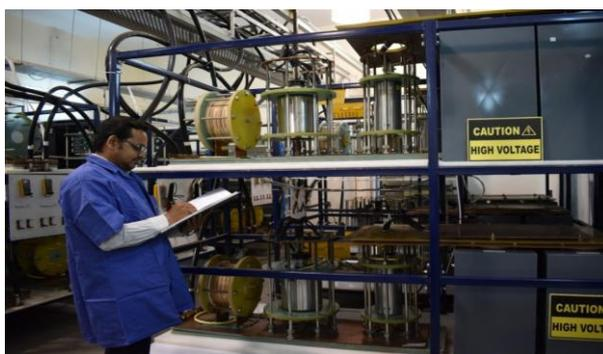
Fig 6: 400 kJ Capacitor modules at ARDE
