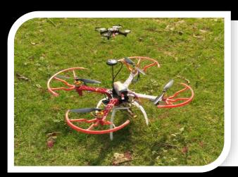
Two Drones. One enabled with auto-stabilisation mode using Pixhawk flight controller and other is Pluto X Nano Drone for indoor environment
